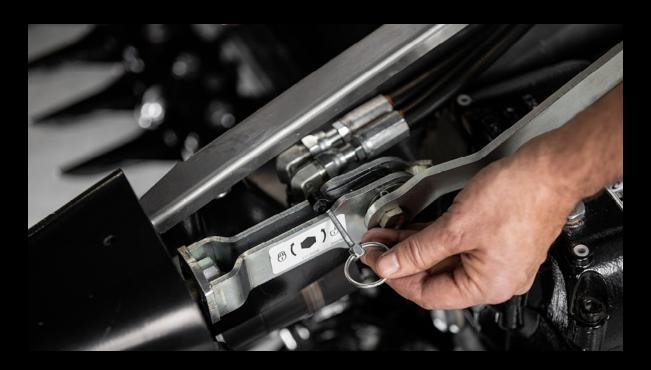
MacDon's Quick Latch End Divider System lets you hook and connect your divider in one move. When using VertiBlade™ Vertical Knives, the standard divider rods store neatly onboard.
