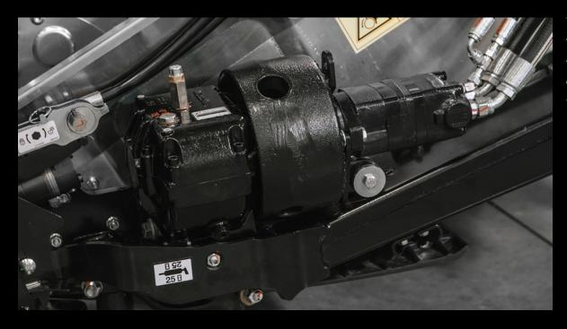
ETDK (Electronically Timed Double Knife) helps reduce header vibration
