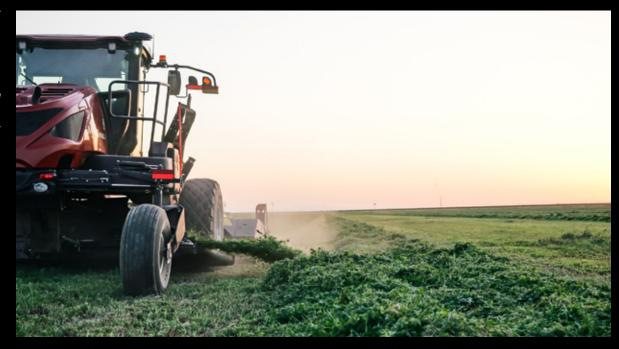
MacDon's optional Double Windrow Attachment (DWA) lets you achieve the ultimate windrow when paired with a rotary disc header. This option is ideal for keeping today's large forage harvesters working at capacity, allowing operators to combine up to three passes into a single windrow. That translates into significant time and fuel savings in the field. The DWA is just another innovative solution that lets you get more with MacDon.
